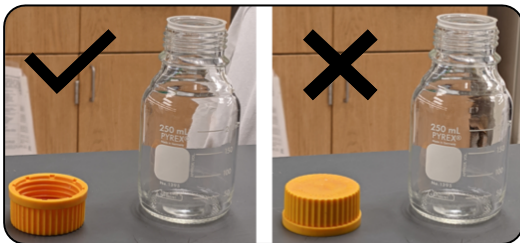
Figure 8. Properly placing a lid upside down (left image) vs improperly placing a lid right side up (right image)
