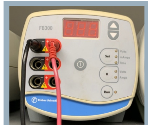
Figure 18. Photo of a Fisher Scientific FB300 power supply with wires connected from the positive and negative nodes of a gel electrophoresis chamber.
