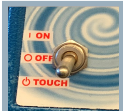
Figure 7. Photo of the on/off/touch switch on a research-grade vortexer..
